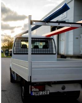
Armaton MP LongGoods makes it possible to transport long goods in a safe and secure way on light commercial vehicles (LCV). With Armaton MP LongGoods, the load is safe throughout the transport and the risk of damaged goods is minimized.
