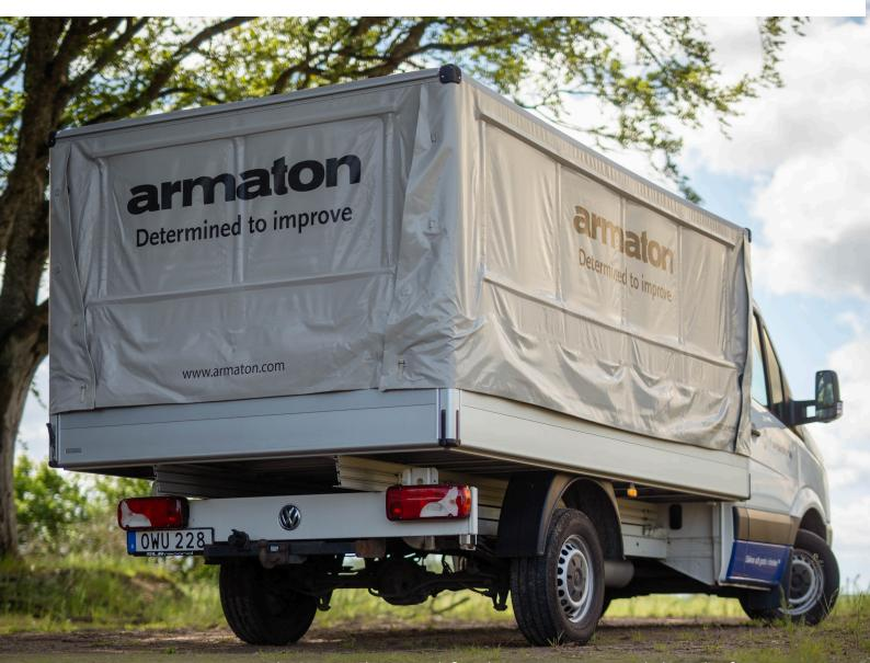
Armaton MP Tarpaulin Kit is designed for the Armaton Modular Platform, making assembly and disassembly easy. The stand mounts into existing pillars on the dropside, and the tarpaulin attaches directly to the dropside without exterior straps or buttons.
