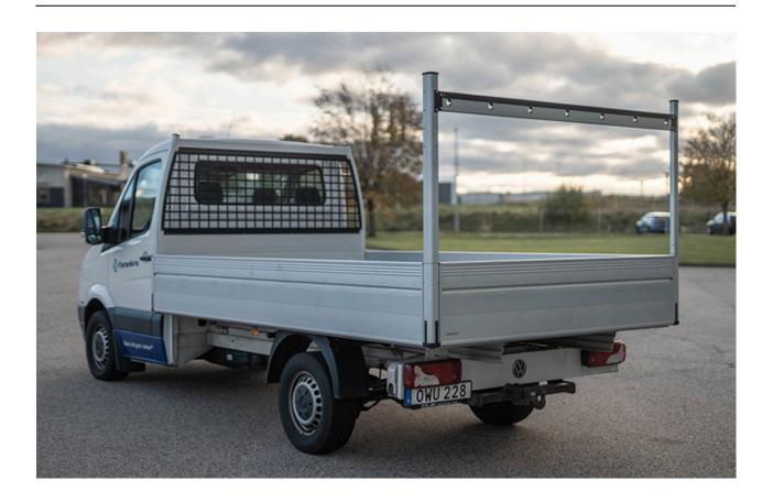
Armaton MP LongGoods makes transporting long goods vehicles safe and secure. It easily mounts into the dropside and front wall, providing a complete solution.
