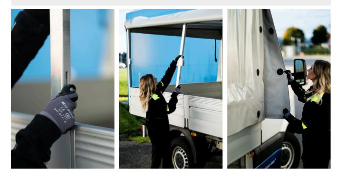
With side pillars the tarpaulin can be equipped with removable side bars to make loading and unloading easier from the side. Easy to close with hidden straps and magnetic locking.
