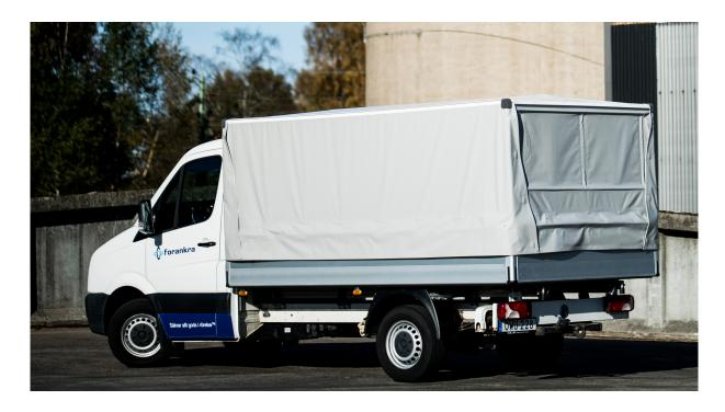
Armaton MP Tarpaulin Kit includes a tarpaulin with aluminum stand designed for Armaton Modular Platform. The kit is easy to assemble and disassemble as the stand mounts into existing pillars on the platform and the tarpaulin attaches directly to the dropside without need for exterior straps or buttons.
