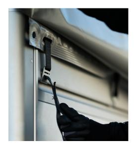
The dropside design makes it possible to mount the tarpaulin directly to the dropside without need for exterior straps or buttons.
