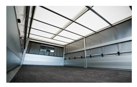
Armaton MP Tarpaulin has light-permeable roofing which provides more light to the load area. The transparent screen against the cab window provides overview of the loading area.
