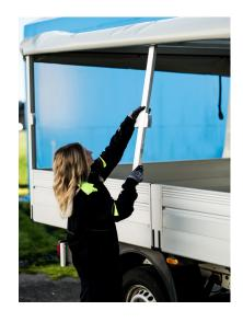
For platforms with side pillars the tarpaulin can be equipped with removable side bars to make loading and unloading easier from the side.
