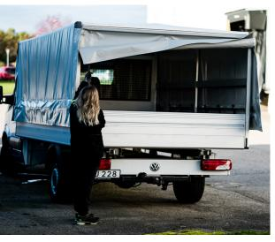
The rear curtain can be a rolled up. Roll-up function for the sides can be added.
