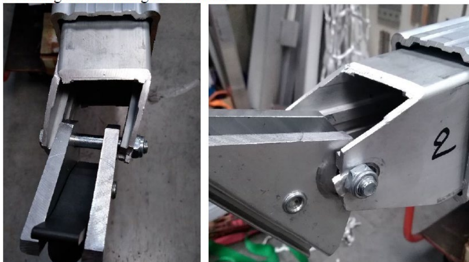
Cracking and breaking at \approx 800daN
