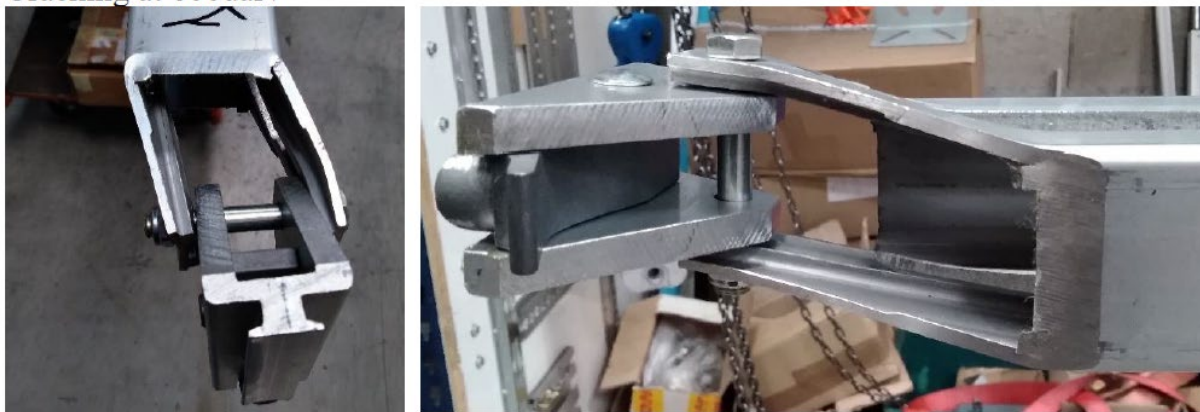
Cracking and breaking at \approx 800daN
