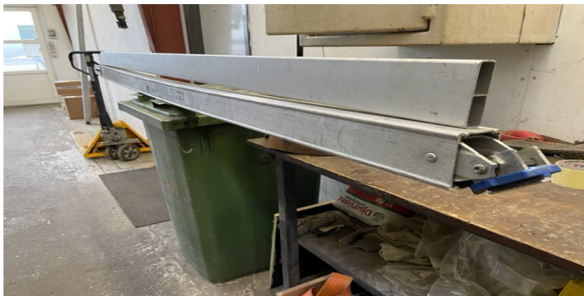
No deformation of the sliding but deformation of the tube.
